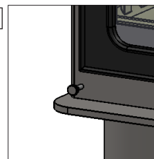
Air vent control
